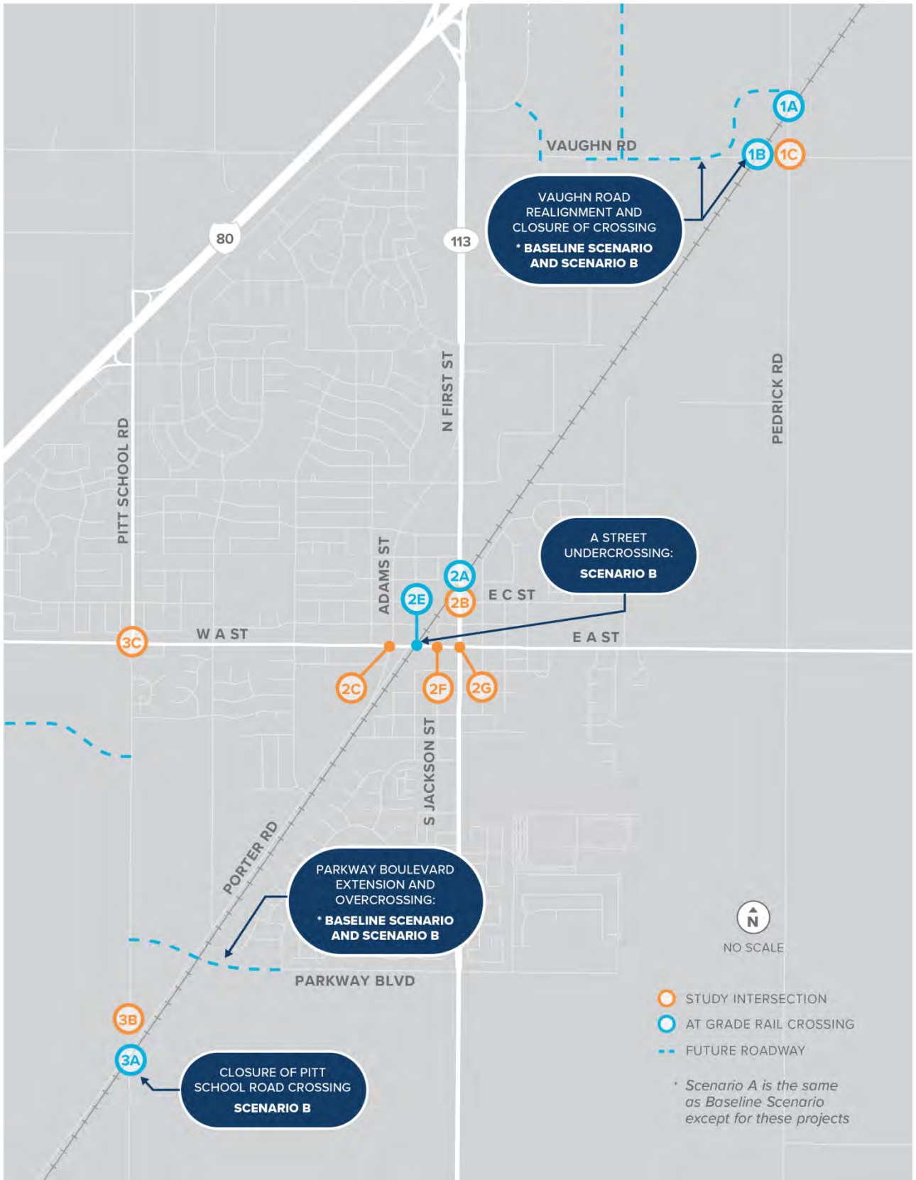
FIGURE 5. ROADWAY IMPROVEMENTS ASSUMED IN EACH FUTURE SCENARIO
