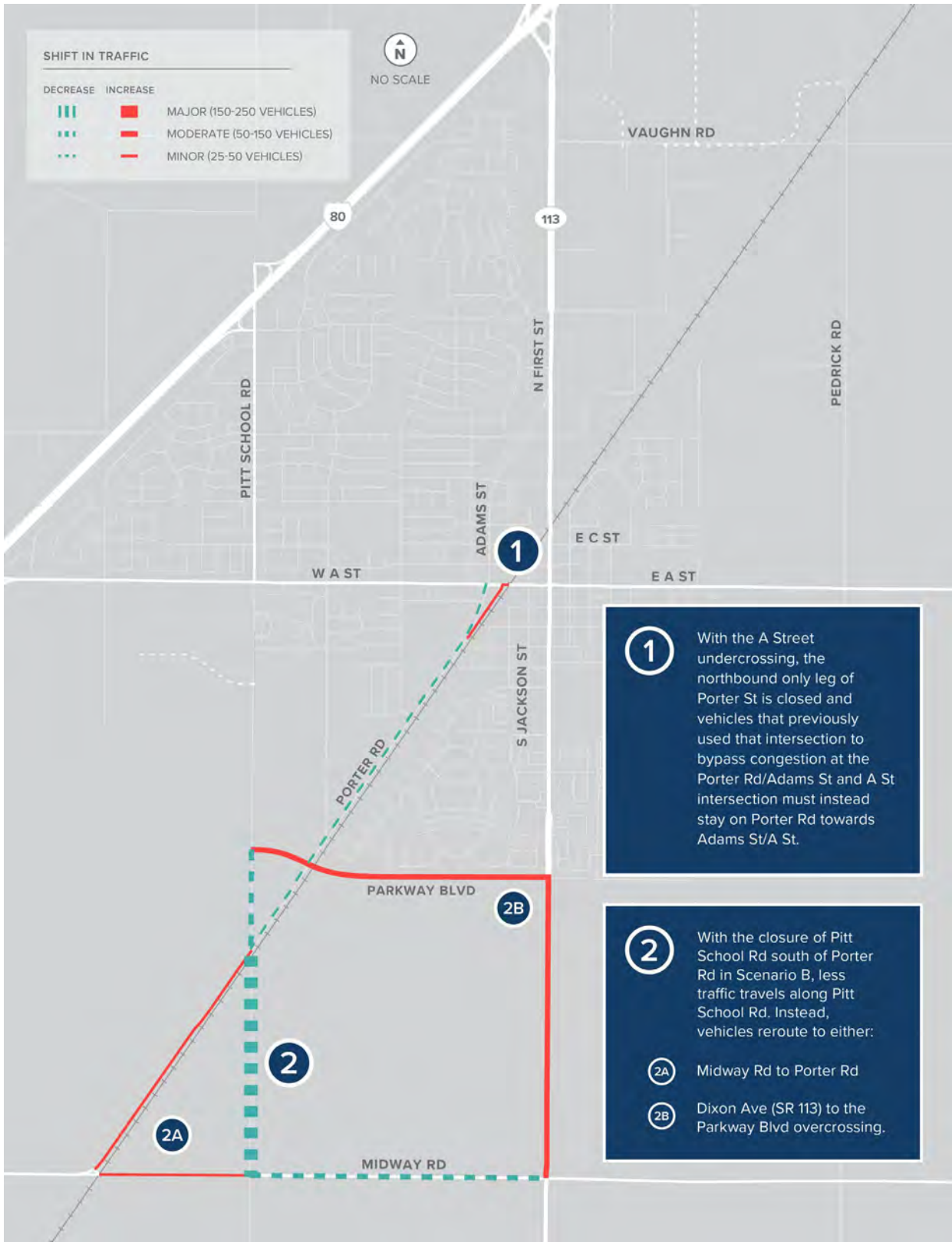
FIGURE 4B. SCENARIO B: SHIFT IN PEAK HOUR MOTOR VEHICLE VOLUMES COMPARED TO BASELINE
