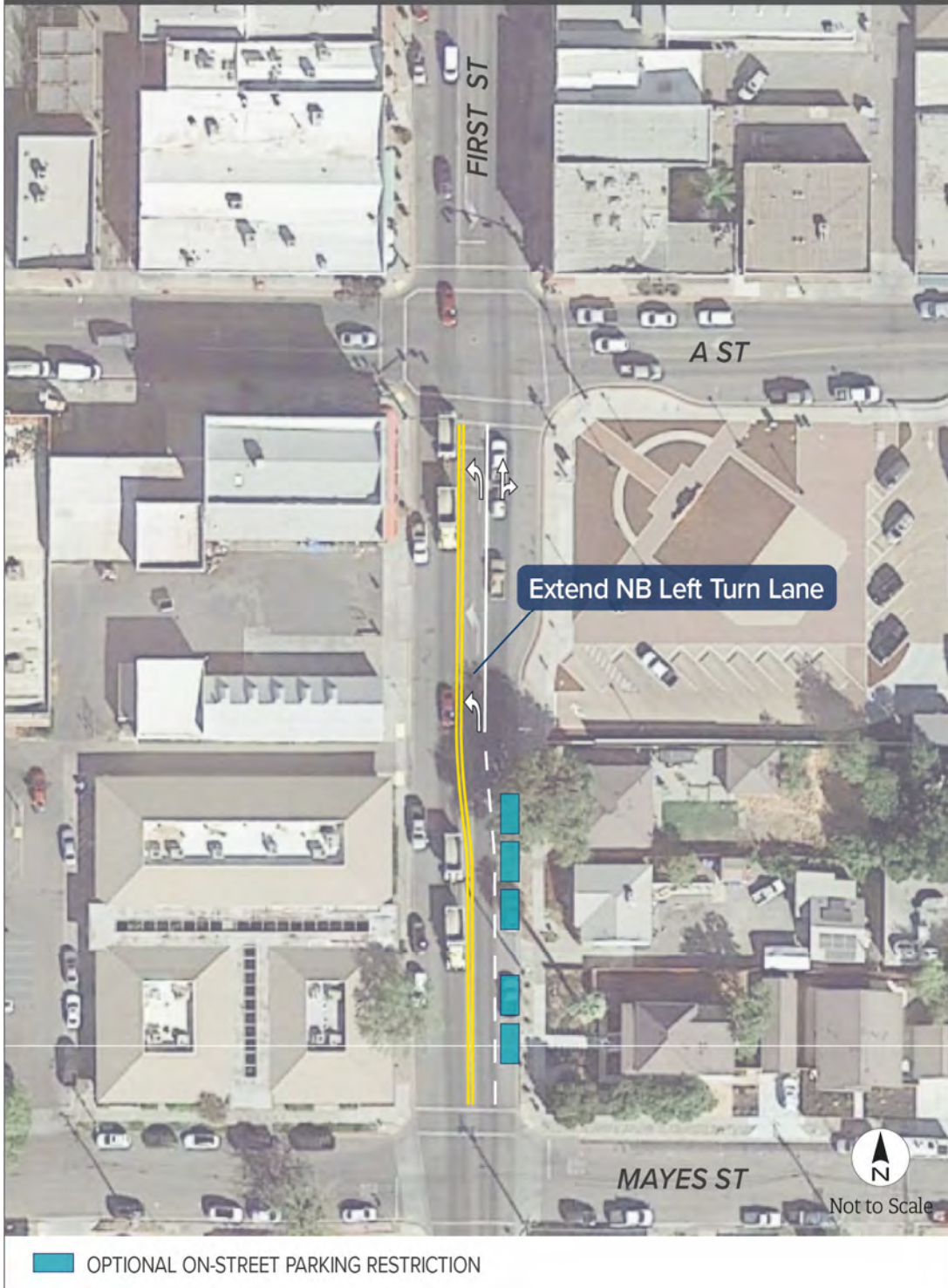
FIGURE 10. OPTIONAL MITIGATION FOR FIRST STREET QUEUEING
