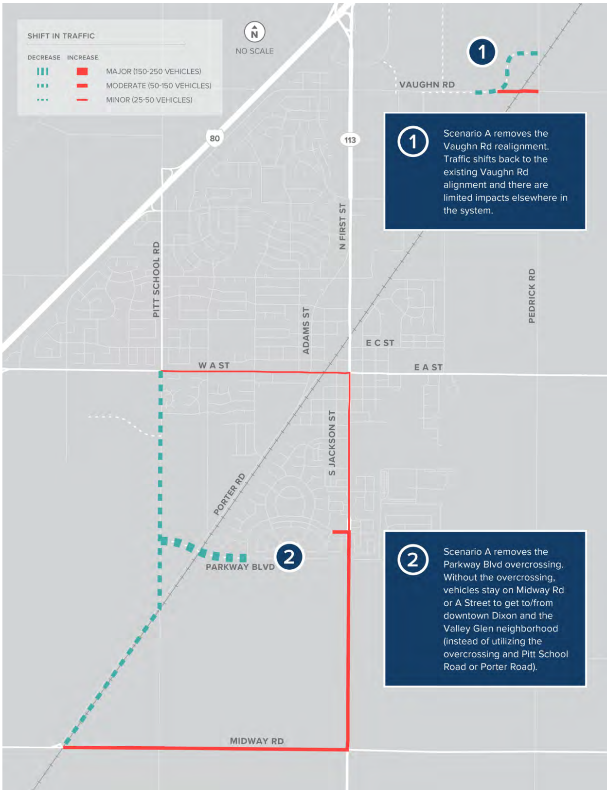
FIGURE 6A. SCENARIO A: SHIFT IN PEAK HOUR MOTOR VEHICLE VOLUMES COMPARED TO BASELINE
