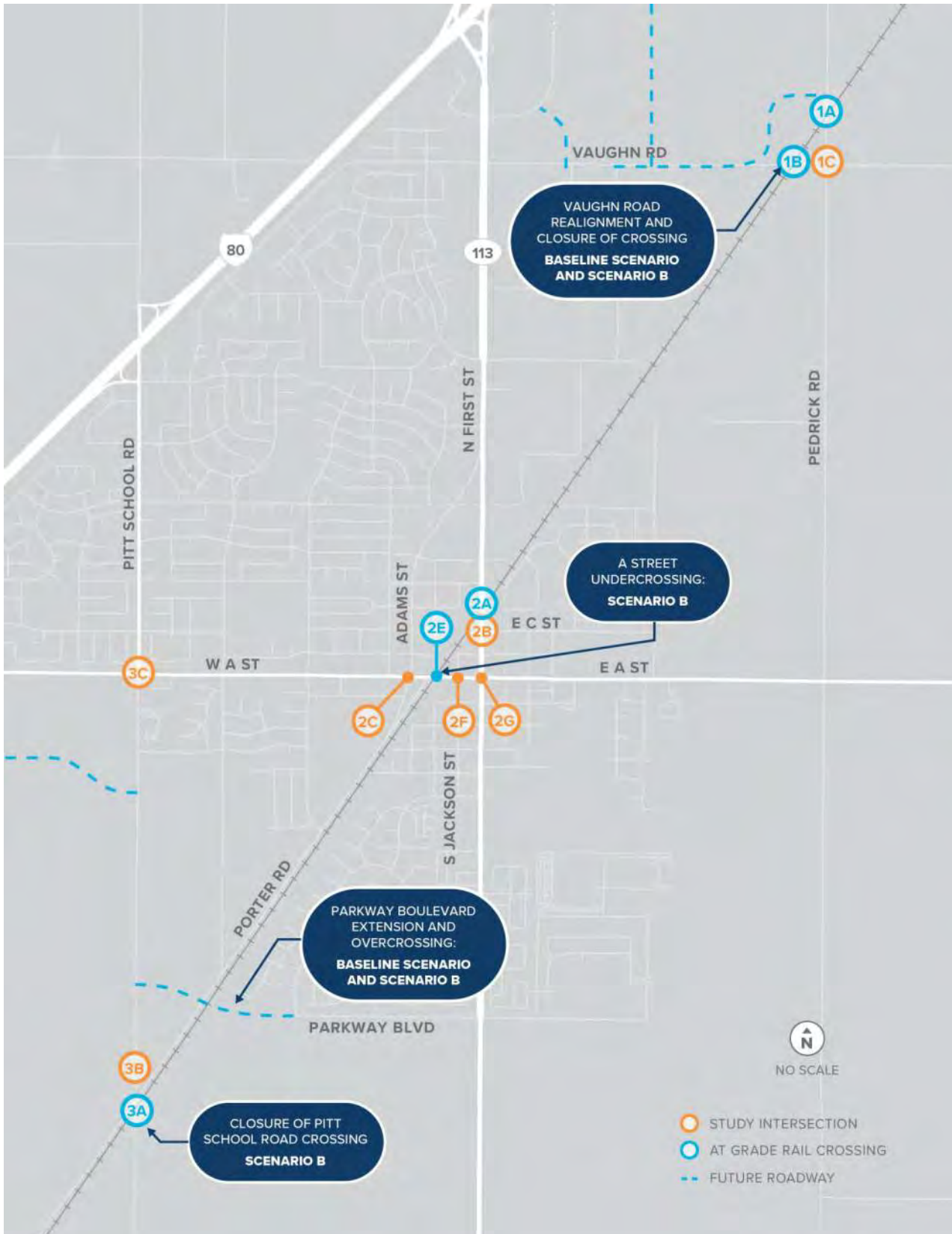
FIGURE 3. ROADWAY IMPROVEMENTS ASSUMED IN EACH FUTURE SCENARIO
