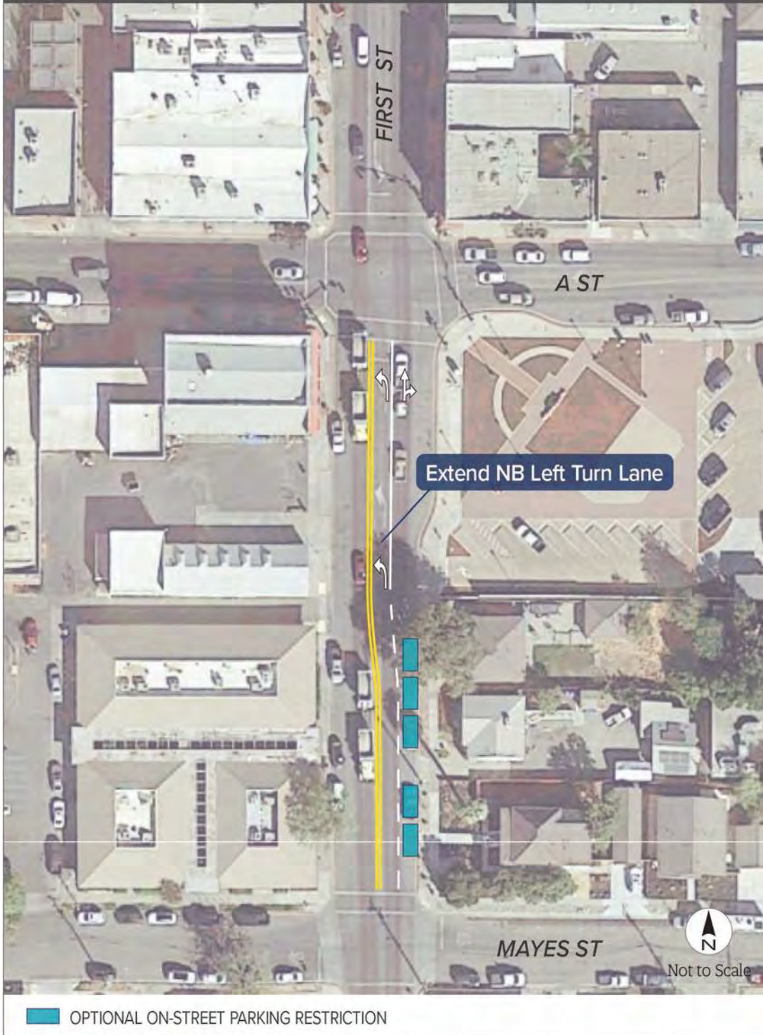
FIGURE 9. OPTIONAL MITIGATION FOR FIRST STREET QUEUEING
